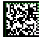
Quiet zone violation
