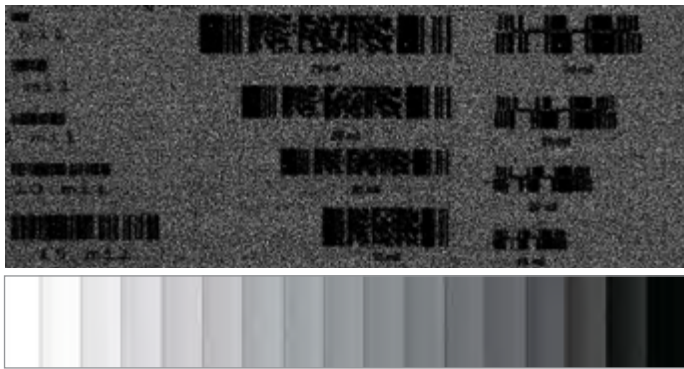
Image taken with conventional 8-bit sensor
