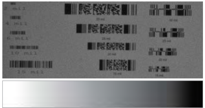
Image taken with DataMan 470 12-bit sensor
