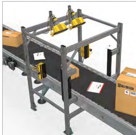
Multi-sided scan tunnel
