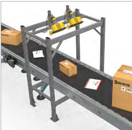
Single-sided scan tunnel
