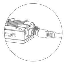
2. Connect the Ethernet cable's RJ-45 connector to a switch/router or PC, as applicable.
